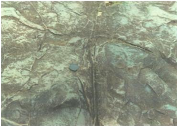
Plate 9. Joint pattern typical of the newer basalt that acts as a dyke (Note the micro faulting)
